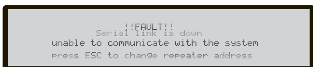
Figure 51 Display "the repeater link is down"
